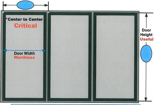
\*Center to Center is measured as the distance from the upper left corner of the 1st door to the upper left corner of the 2nd door.
