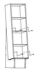
Using (4) #8 x 1.5" screws, attach bin to floor stand
