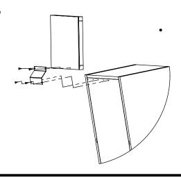
Using (4) #8 x .5" screws, attach Sign (item 8) and Bracket (item 7) to Bin.
